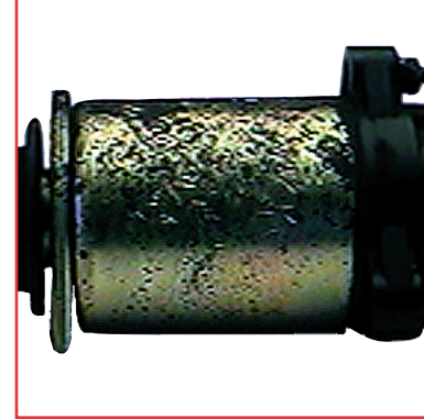
Solenoid cover has been struck repeatedly with a hammer or some other foreign object.
