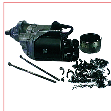
Exploded commutator and brush debris.
