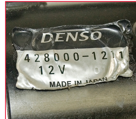
ID tag has been overheated and has shrunk. This is a sign of excessive heat.
