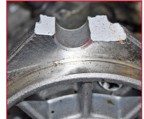
Starter to engine mounting bolt hole broken off due to mishandling, improper installation, or over-torquing of the engine bolt.
