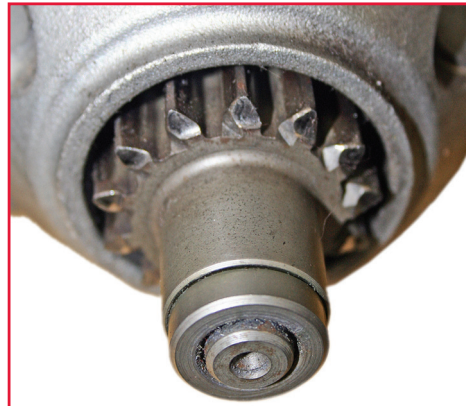
B.) Moderate case of pinion re-engagement.
