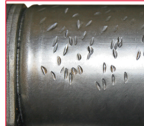
Solenoid cover has been struck repeatedly with a hammer or some other foreign object.
