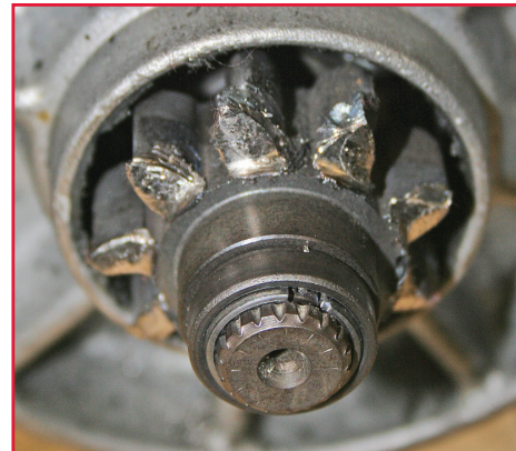
C.) Extreme case of pinion re-engagement.
