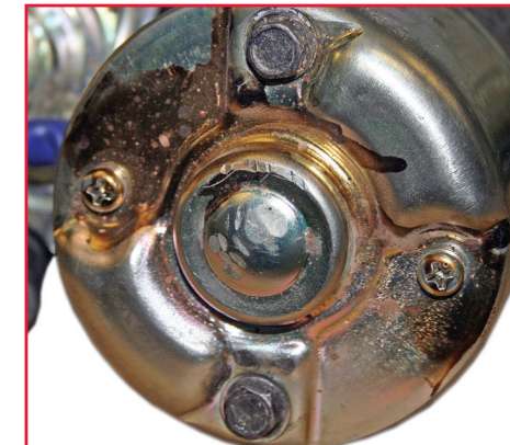
Melted insulation on the starter end housing thru bolts. This is a sign of starter abuse (overheated).
